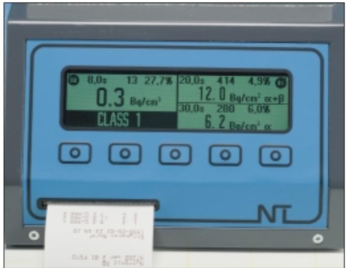
A measurement in auto-alpha mode with the NT200. In the right windows alpha activity has been registered. The display clearly indicates this and shows the alpha and beta results separately.
