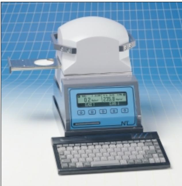
*The optional external keyboard can be used to document the smear samples, adding comments where needed.*
